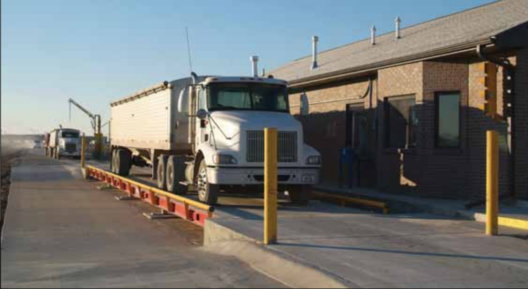
Line of incoming trucks await processing, with 80-foot Fairbanks Truck Scale in foreground and Gamet truck probe in background.
