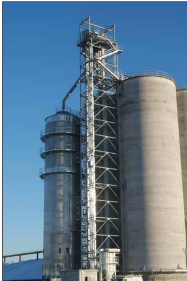
New 7,000-bph Zimmerman grain dryer served by 15,000-bph Intersystems wet and dry legs.
