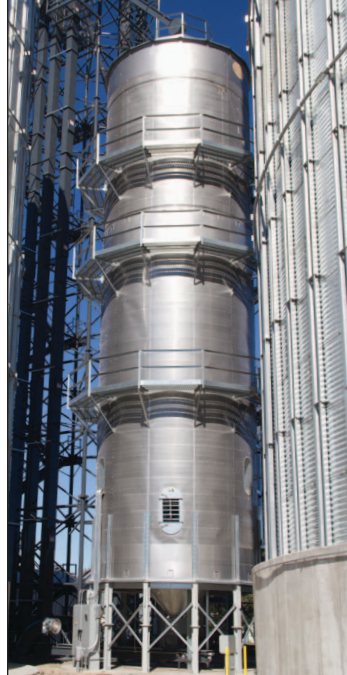
3,000-bph GSI tower dryer.
