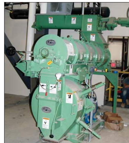
CPM Model 1116 pellet mill runs 7 tph of pellets. The line also includes a Geelen counterflow cooler and CPM screener and crumbler.
