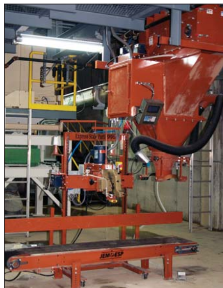
Express Scale bagging line will bag between 15% and 20% of the research mill’s output for use at the OARDC or outlying stations.
