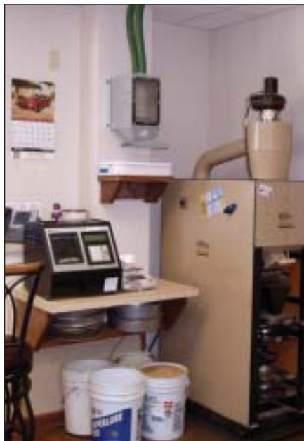
Grain quality lab includes a DICKEY-john GAC 2100 moisture tester and an MCI Kicker dockage tester.
