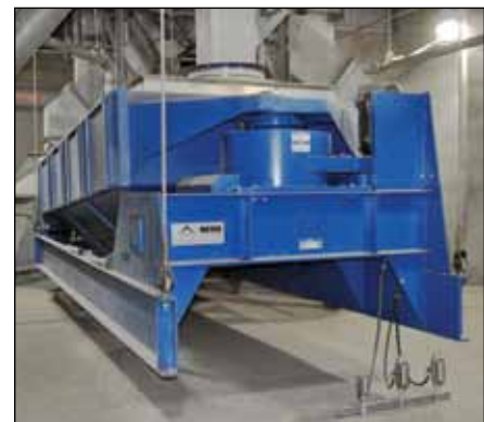
Carter-Day indent cylinder separator (top) and Rotex vibratory screener (bottom) are among the cleaners used to clean grain to export standards.
