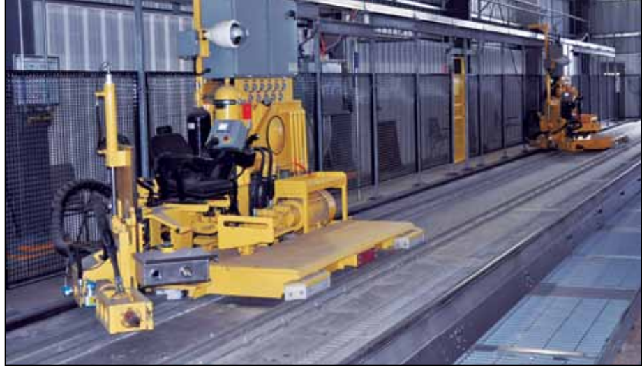
Two robotic Calbrandt railcar gate openers service trains inside the facility receiving shed, which includes a pair of 60,000-bph mechanical receiving pits.
