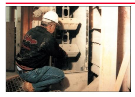
Lightweight Maxi-Tuff<sup>10</sup> buckets cut chain and sprocket wear because they weigh 80% less than the cast iron buckets previously used.
